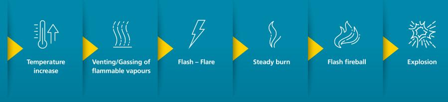
As lithium-ion batteries are made of a series of cells, the thermal runaway will typically start in one cell before expanding in a domino effect through the adjacent cells.
